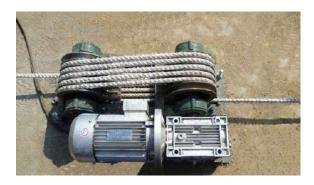
The scraper type manure collection machines is designed for A frame cage systems which has manure pits under the cages.
