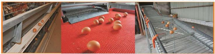
Automatic egg collection unit made of galvanized sheet and apparatus produced by our advanced own production machines. The egg bands and lift engine powers are 0.75 -1.50 HP.
