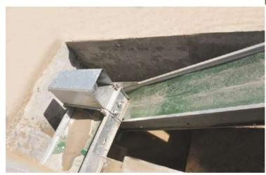
Vertical manure conveyor: The rubber band in thickness of 6 mm including the cord cloth running on galvanized pipes at galvanized construction and the front rear rollers, reducer engine.
