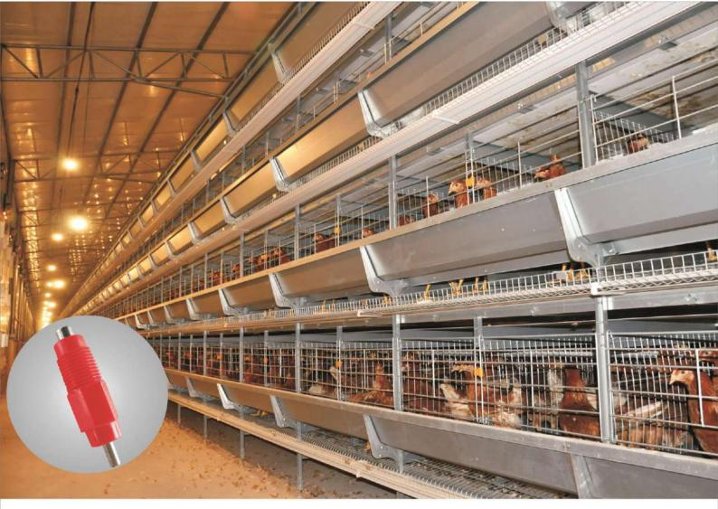
Watering system is consisting of PVC material square shape pipe, nipple drinkers, which is made of plastic and stainless steel in red color, in each section and the bottom plastic drop catcher in V shape. and all nipple drinkers will be fitted with the square pipes already and packed by carton and plastic bags outside for protection before shipment.
