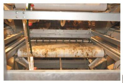
Manure is cleaned and discharged by the Polypropylene (PP) manure belts of 1.10 mm thickness. These PP belts are located underneath every tier and row of the cages and towed by drive reducer engines to clean the manure in a flawless way.
