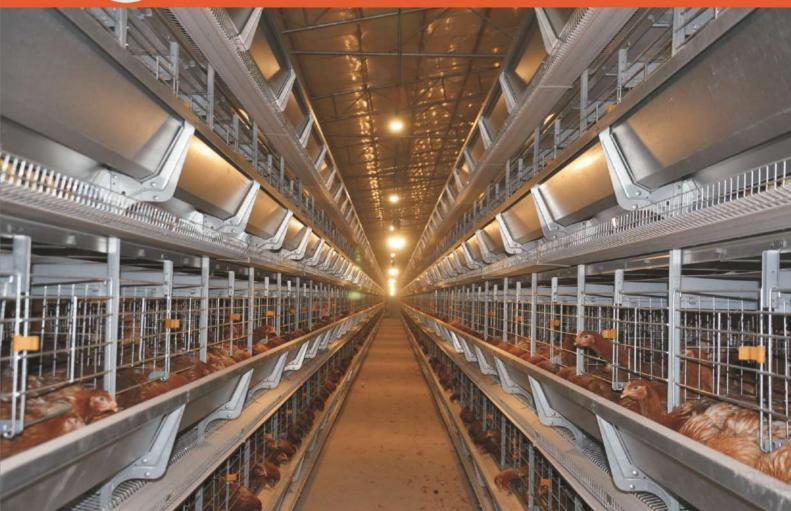
The H frame layer cage system construction and the sections of cages are produced of galvanized sheet and hot dipped galvanized wires bearing ISO 9001 Quality Certificate. The material is high standards. It is becoming the most popular and good choices to the poultry farms all over the world.
