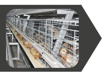
The height of the trough is easy to adjust: The height of the trough of the TechEasy broiler cage can be adjusted at will to ensure that chicks of different ages can eat normally.
