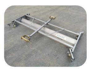
The manure dropping from the cages in the manure pits, and the scraper can collect the manure from manure pits to the outside of house.
