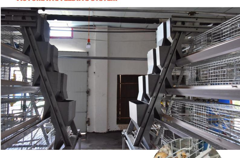
Feeding hopper is connected by rivets without welding, making it more durable.
