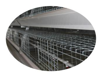
Both the cage meshes and cage stands are made by hot galvanization steel, which ensure the chicken cage can withstand the corrosion of chicken manure for a long time, the service time of the chicken cage can reach more than 15 years.
