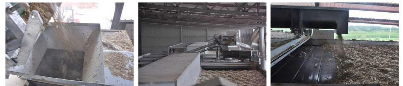
DISTRIBUTION DEVICE: Even distribution of manure on the drying plate leads to uniform and efficient drying
