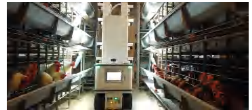
Chicken house inspection robot(SHEEPDOG)
