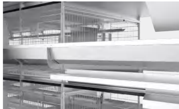
Deepened V-shaped feed trough avoid feed waste caused by feed lifting
